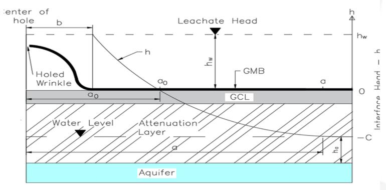
Fig. 1. Schematic showing extent of wetted distance beneath a holed wrinkle.
