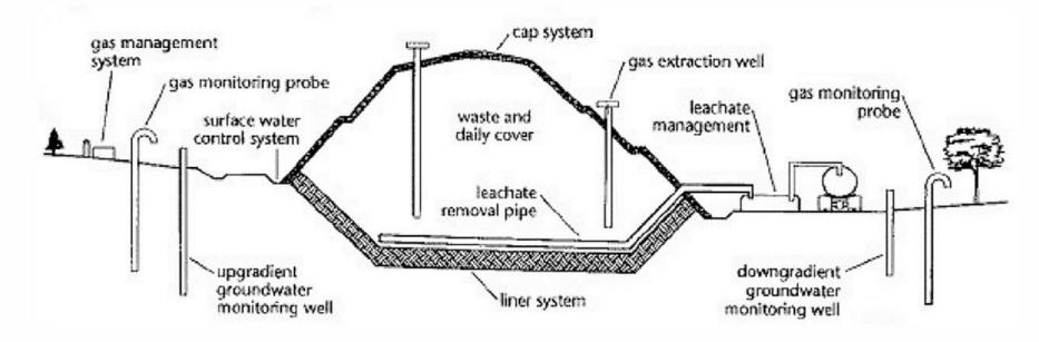
A typical schematic design of an engineered landfill with a full leachate and gas management. Source: UNEP (2002)
