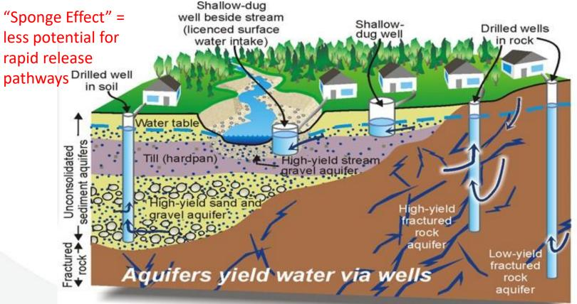
Fractures = much greater potential for rapid release pathways and high flow velocities
